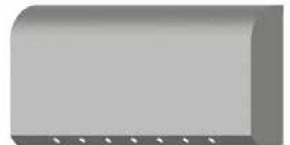
(7) 3/4 in. light holes on 45° face IC172007-21
