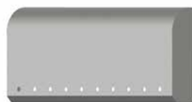
(10) 3/4 in. light holes on 45° face IC172005-21
